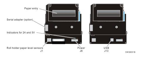
Figure 1 • Printer Exterior, Rear View
